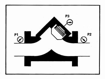
Fully Open: The pressure differential across the valve (P1 minus P2) is equal to the spring force in the fully open position.
